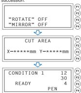
The plotter is now ready to receive data for cutting or plotting. If the interface or command settings have not been made, make these settings before sending the data. If the settings have been made, perform pen adjustment. When the pen adjustments have been made, the plotter is ready to start cutting. Send the cutting or plotting data from the application software.
