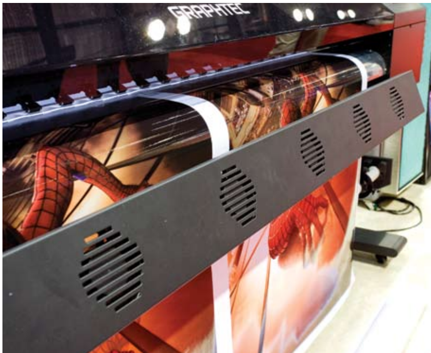
Fig. 5: From this view, you can see the dryer unit, which comes standard with the printer and spans the maximum width the printer can produce.
