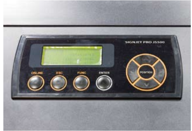
Fig. 2: All the printer's functions, including heater- and dryer-temperature settings, are handled through the LCD control panel. The well-arranged buttons facilitate menu navigation and parameter setting.
