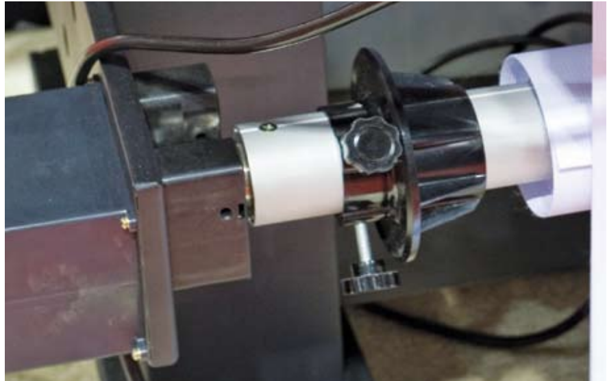
Fig. 4: Though the images aren't taped to the take-up roll, you can see the path the media takes. The large, core ends can easily handle heavy media.
