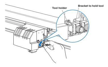
While pushing up the tool holder, push until its flange completely touches the upper part of the holder.
