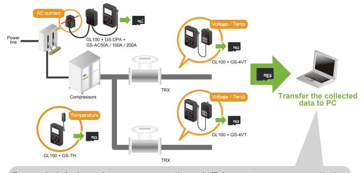
Easy analysis for improving power consumption and efficiency at compressor operation!
