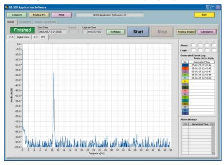
The frequency axis changes automatically according to the Current sampling interval setting.
