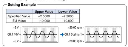
setting function that enables all the SPAN settings for the group to be set simultaneously to the same values.
