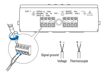
Use the provided screwdriver to loosen the terminal screws. Insert the cables in the terminals, and then tighten the screws to hold the cables in place.
