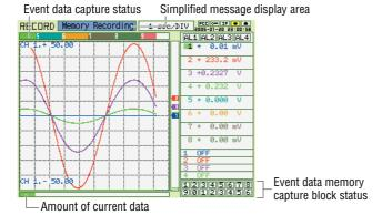
During data capture, the memory blocks at the bottom right of the screen light red in succession to indicate the capture status.
