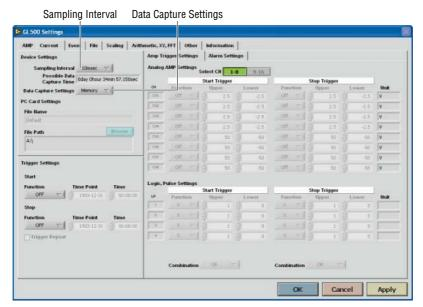
Make the "Sampling Interval" and "Data Capture Setting" settings. In the screen displayed above, the following settings were made.
