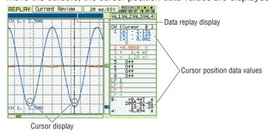
(3) Press the TIME/DIV key to change the time axis of the displayed waveform and make the waveform easier to view. If the TIME/DIV key is pressed twice in succession, the waveform being displayed will be stopped.
