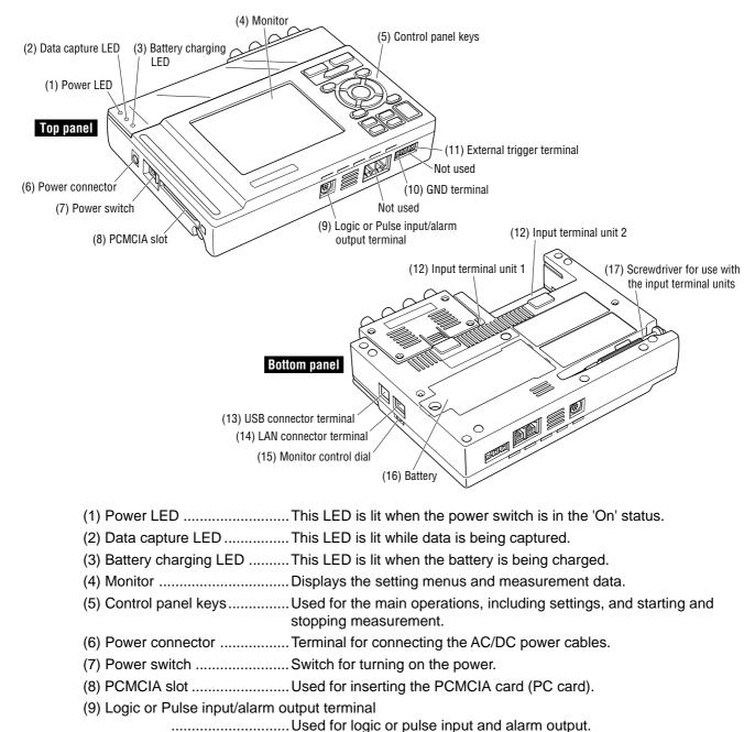
(10) GND terminal......Connects the main unit to ground.
