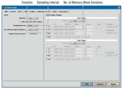
Make the "Function", "Sampling Interval", and "No. of Memory Block Divisions" settings. In the screen displayed above, the following settings were made.
