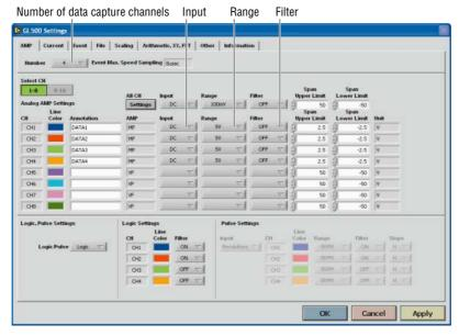
Specify the number of data capture channels for "Number". Use the number of input signals for this value.
