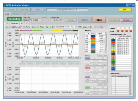
Y Axis Range 1, 2: Y-axis scaling can be displayed for two channels.
