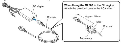
(2) Connect the output side of the AC adapter to the power connector on the GL500.
