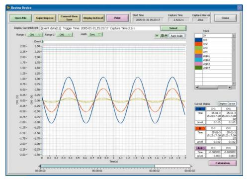
Click the "Superimpose" button to display the "Select File to Superimpose" screen.
