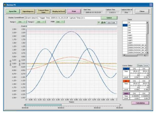
Click the "Superimpose" button to display the "Select File to Superimpose" screen.
