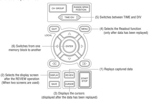
(1) REVIEW key...... Use this key to replay data after the measurement operation has been completed.
