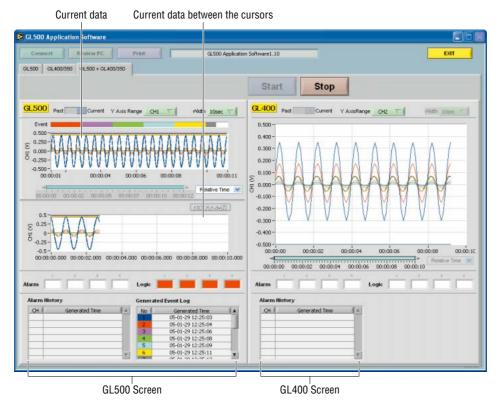
Data capture start and stop operations can be performed using this screen.
