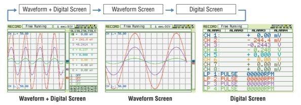
Waveform + Digital Screen: Both waveform and digital data are displayed together. Waveform Screen: Only waveforms are displayed over the entire screen.
