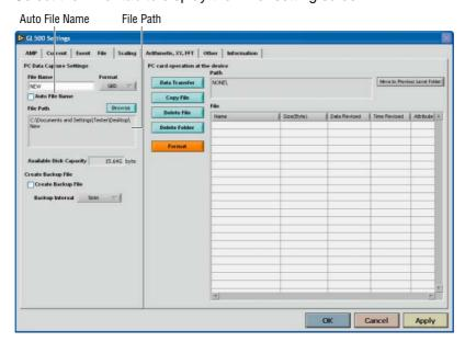
Make the "Auto File Name" and "File Path" settings for data capture at the PC. In the screen displayed above, the following settings were made.
