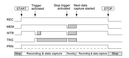
• The Trigger Function setting is Memory, both the Start Condition and Stop Condition settings are On, and the Record Function setting is Memory:
