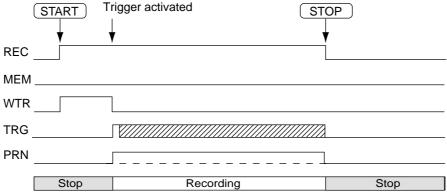
• The Trigger Function setting is Record and both the Start Condition and Stop Condition settings are On:
