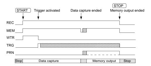
• The Trigger Function setting is Memory, both the Start Condition and Stop Condition settings are On, and the Record Function setting is Direct:
