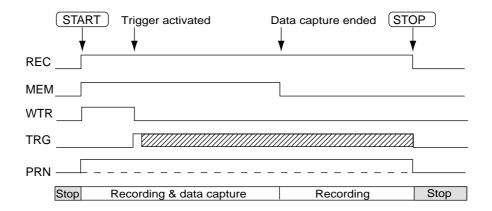
• The Trigger Function setting is Memory, the Start Condition setting is On, the Stop Condition setting is Off, and the Record Function setting is Memory:
