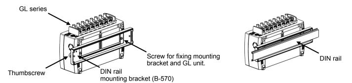
GL series can be mounted to DIN rail using mounting bracket B-570. The mounting bracket is fixed to rail by thumbscrew.
