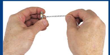
Pull Knot Tight into Hole
